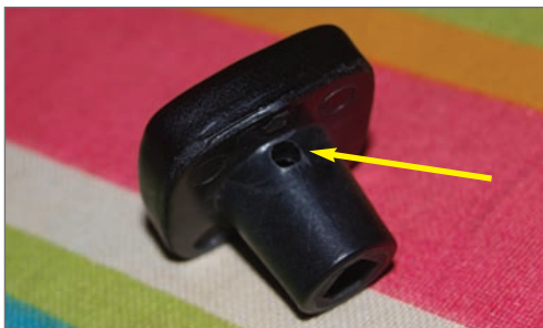
Picture 5 Hole under the knob for releasing the spring clip
