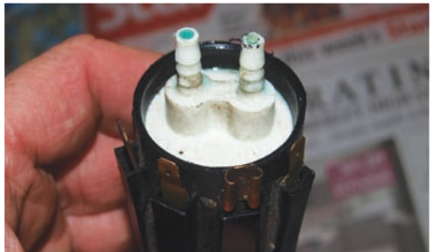
Picture 9 Switch removed, note connections are not all the same as the replacement in picture 1
