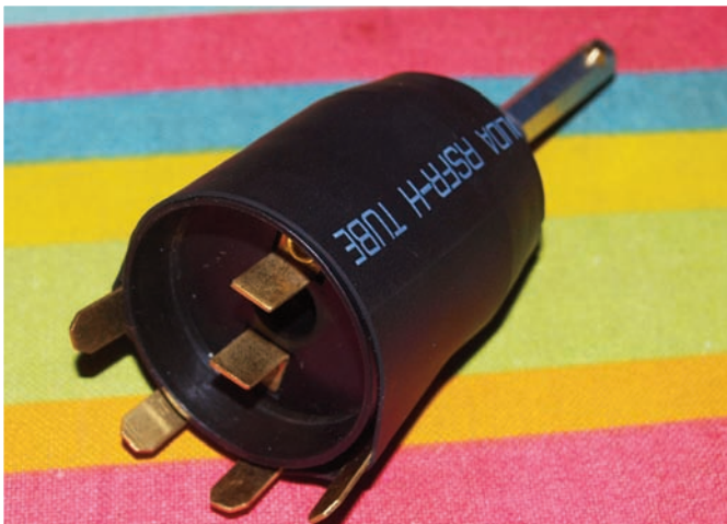
Picture 1 TR6 wash wipe switch which is close to the Original.
