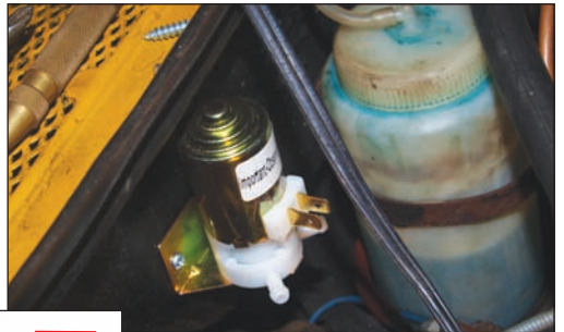
Picture 15. Washer pump mounted on the bulkhead
