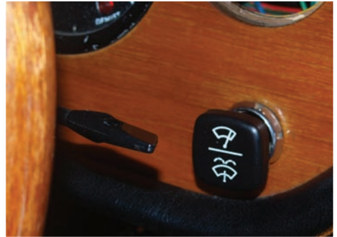
Picture 19 Assembled and working, I even replaced the knob as the logo had worn of the old one.
